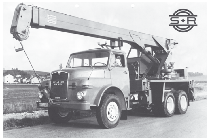
Telescopic autocrane MT 16 with a maximum lifting force of 10 tonnes from the 70's
